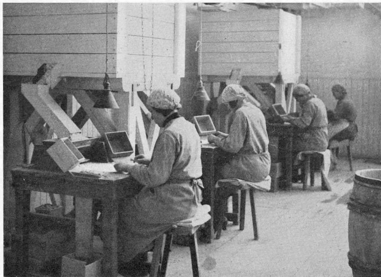
FIG. 14. Female workers hand-sorting small pieces of cryolite at the "picking machine" (table with conveyor belt).
